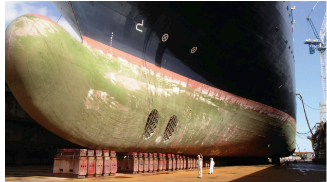
Despite current antifouling measures, removal of slime and other marine organisms still incurs significant costs for the shipping industry. Image: Michael Elleray
