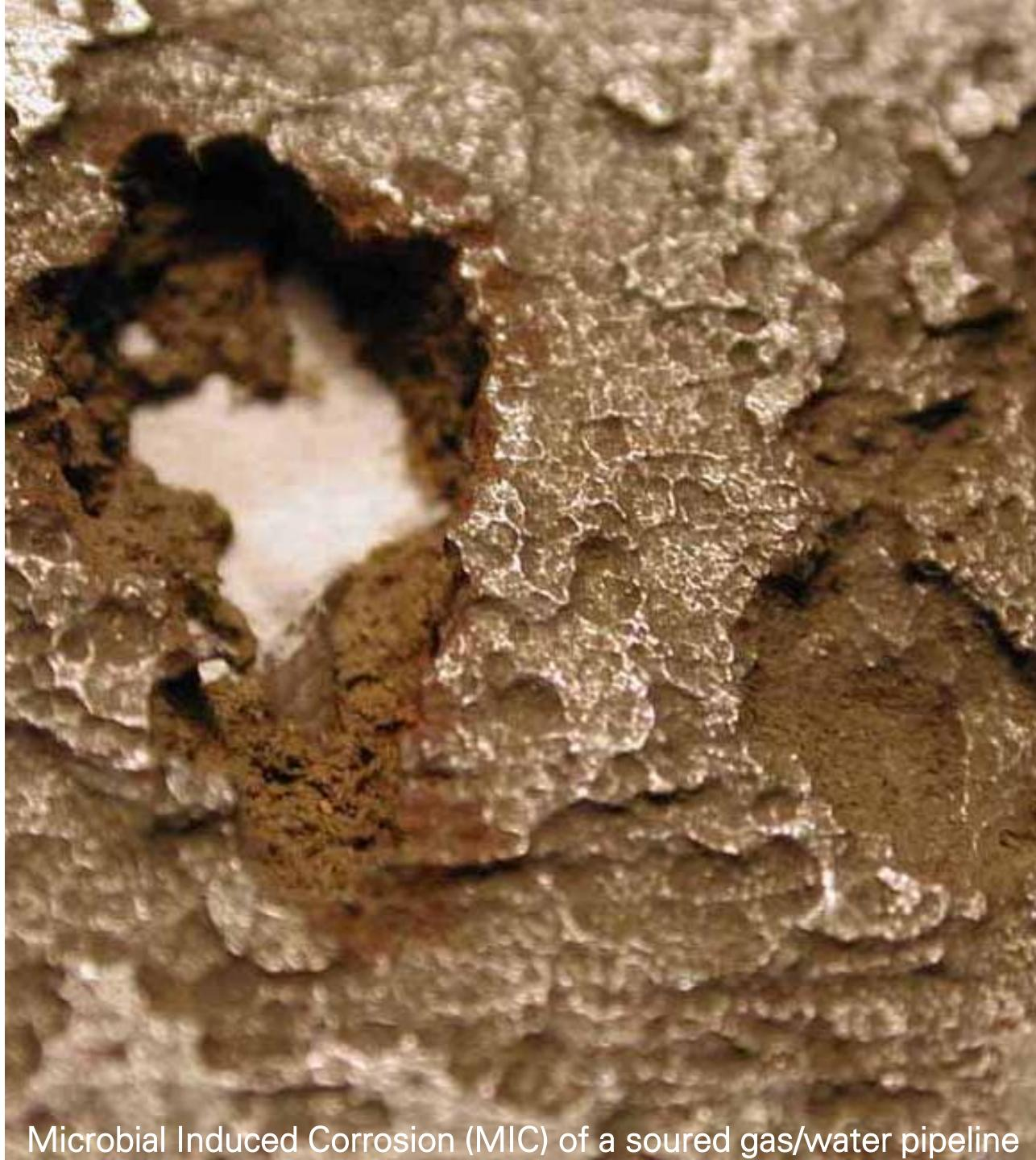
Microbial Induced Corrosion (MIC) of a soured gas/water pipeline
